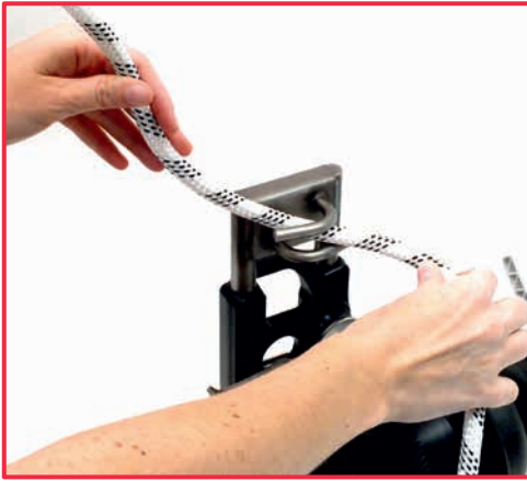
5. Pass the primary rope inside the pins.
