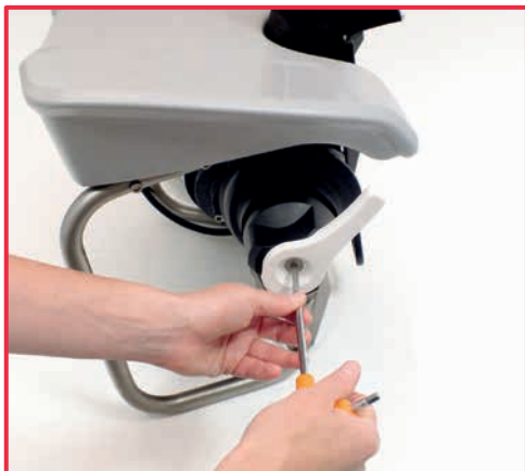
1. Remove and save the knob screw and install the control lever using the screw provided, using an allen key n°5.
